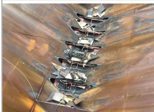
Gate & Hogback replacement inside the cargo holds of the S/S Philip R. Clarke while in lay-up
