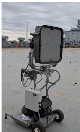
An LRAD (Long Range Acoustic Device) set up on the weather deck of the Cape Douglas.
