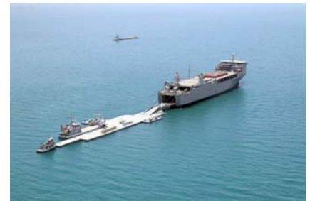
M/V Cape Ray with her stern ramp lowered onto the Roll-On/Roll-Off Discharge Facility preparing for cargo operations
