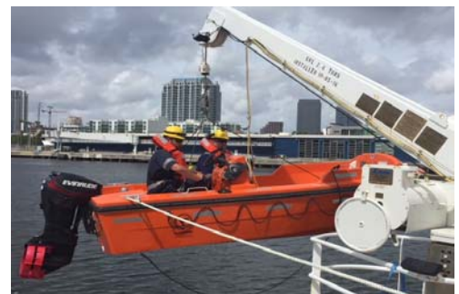
ABS Auditors test the Fast Rescue Boat during the audit
